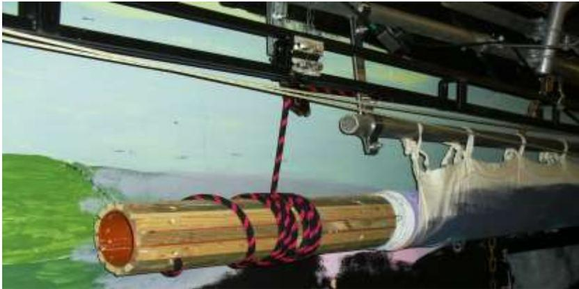
Does anyone know why our backcloth rollers looks like this? The middle is a 4 inch pvc soil pipe with thin wooden strips screwed around the outside. This one is actually two pipes joined together making 7.5 metres overall. The other one is only 6m long
